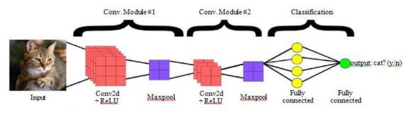
Figure 2. The architecture of a CNN used in the prediction matic flowchart of the build pipeline
